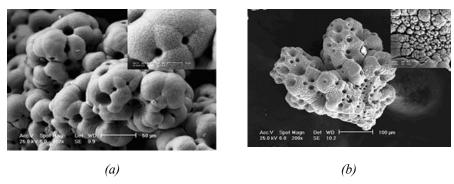
Fig. 3 SEM microphotograps of cobalt powder particles deposited at  $j_{L(Co)} = 770$  mA cm<sup>-2</sup> onto glassy carbon electrode; (a) the agglomerate and detail of surface, (b) spongy-like particle with detail of surface.
