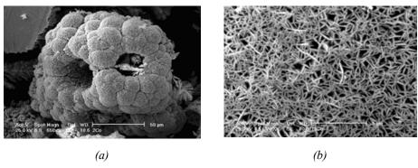
Fig. 2. SEM microphotograph of the (a) compact agglomerate, (b) surface of cobalt powder particle electrodeposited onto glassy carbon at  $j_{Co} = 500 \text{ mA cm}^{-2}$ .
