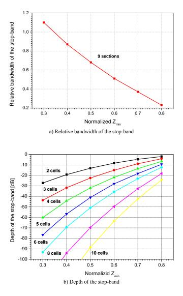
Fig. 4. Curves for cells with 9 sections versus normalized  $Z_{min}$  (i.e.  $Z_3 / Z_0$ )
