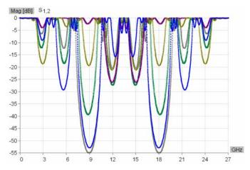
Fig. 2.  $S_{12}$  of cascade of four identical cells made of nine sections obtained for five random choices of section impedances.
