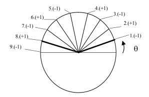
Fig. 3. Position of band-gaps depends on angle (bold lines mark desirable bandgaps) (-1) or (+1) correspond to boundaries of the dispersive polynomial
