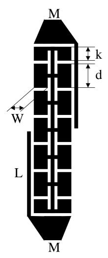
Fig.6- Lay-out of the realized slow-wave band-pass filter (W=1.3mm; d=1.4mm; k=0.8mm)
