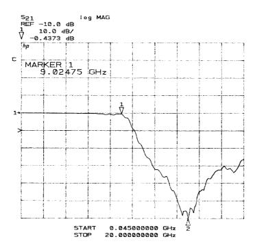
Fig.5b- Measured  $S_{21}$  parameters for the realized low-pass filter with three cells
