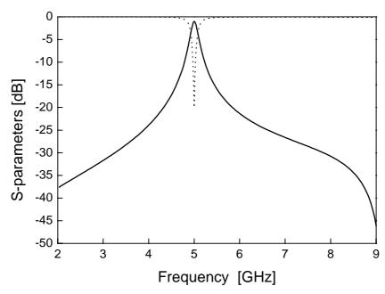
Fig.7- Simulated S-parameters for the proposed structure in Fig.6 ( $S_{2I}$ -solid line;  $S_{II}$ -dot line)
