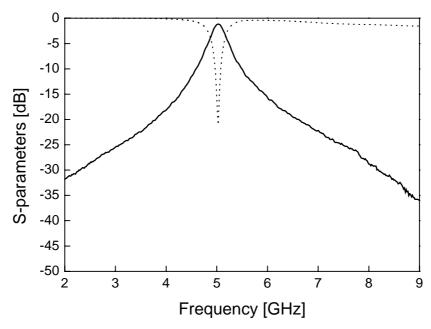
Fig.8- Measured S parameters for the proposed structure in Fig.6 ( $S_{21}$ -solid line;  $S_{11}$ -dot line)
