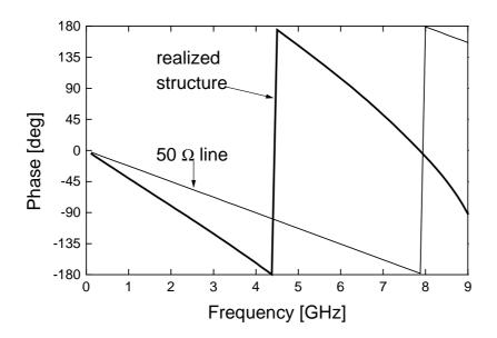
Fig.3-Phase responses of the realized structure with three cells (including the ordinary 50  $\Omega$  lines for the connectors; Fig.2) and the ordinary 50  $\Omega$  line of the same length
