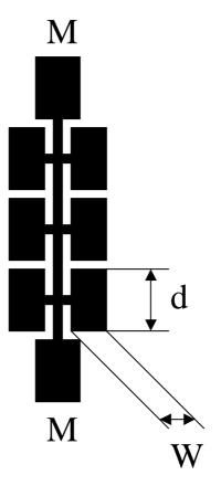
Fig.2- Lay-out of the realized slow-wave low-pass filter (W=1.3mm; d=3mm)
