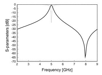
Fig.10- Simulated S-parameters for the structure presented in Fig.9 ( $S_{2I}$ -solid line;  $S_{II}$ -dot line)
