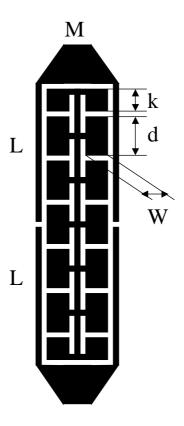
Fig.9- Additional coupling lines around the whole resonator
