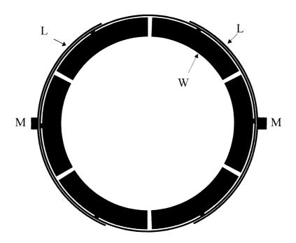
Fig.11- Lay-out of the proposed ring resonator
