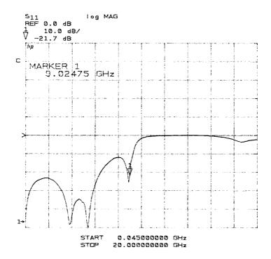
Fig.5a- Measured  $S_{II}$  parameters for the realized low-pass filter with three cells
