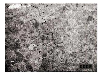
Fig. 4. SEM microphotograph of mechanically then electrochemically polished Cu. × 750
