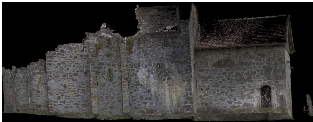
Figure 5: Ortophoto image – north facade view of the monastery church in Slavkovica (point cloud image made by Agisoft Photoscan software)
