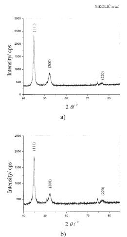
Fig. 5. XRD Patterns of: a) the nickel coating obtained in the presence of the basic brightening addition agent, b) the nickel coating obtained in the presence of both the basic and the top brightening addition agents.
