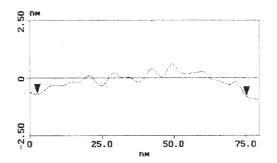
Fig. 4. The line section analysis of the flat part of the nickel coating obtained in the presence of both the basic and the top brightening addition agents. The roughness of the observed surface was 0.220 nm.
