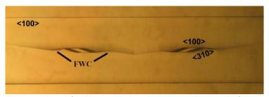
Figure 6. Ridges defined by FWC at the enlarged microphotograph of the first basic pattern with the sides along crystallographic directions <100> and <310> for the etch depth of 54  $\mu$ m.
