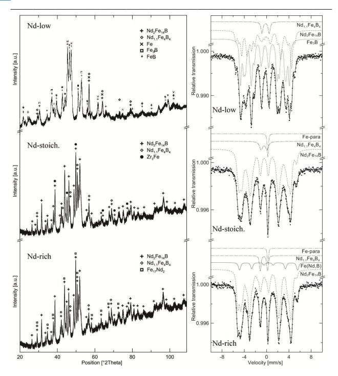
Fig. 2 – X-Ray diffractograms of the investigated alloys
