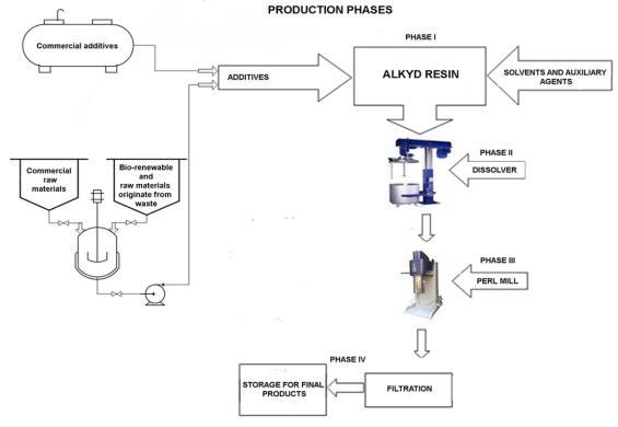
Figure 1. Schematic presentation of production of the alkyd based anticorrosive coatings at industrial level Slika 1. Šematski prikaz proizvodnje alkidnih antikorozionih premaza na industrijskom nivou
