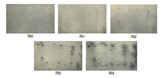
Figure 2. Photographic examples corresponding to ISO 4628-3, to assess the degree of rusting of a painted surface
