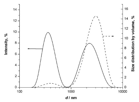
**Fig. 3.** Particle size distribution by dynamic light scattering of TiO<sub>2</sub> solid phase in the medium for Pt deposition.
