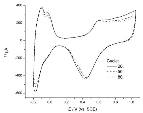
**Figure 2.** Characteristic cyclic voltammograms of Pt supported on C, registered during continuous cycling in deaerated 0.1 M HClO<sub>4</sub> at sweep rate of 100 mV s<sup>-1</sup>.
