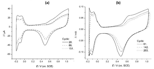
**Figure 1.** Characteristic cyclic voltammograms of Pt supported on  $TiO_2$  at sweep rates of 50 (a) and 200 mV s<sup>-1</sup> (b), registered during continuous cycling in deaerated 0.1 M HClO<sub>4</sub>.
