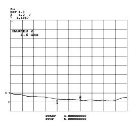
Fig.11b Measured VSWR vs. frequency for omnidirectional antenna with circular polarization and conical radiation pattern
