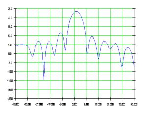
Fig.2c Measured antenna diagram (60 GHz), dBi
