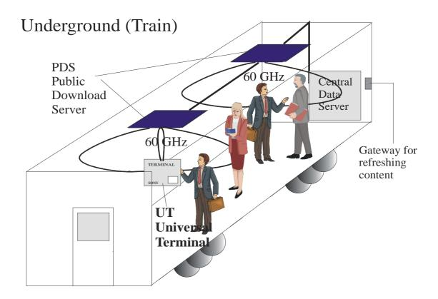
Fig.1c Semi-out-door application for underground. Note that the same approach is for airport, large halls and corporate office scenario
