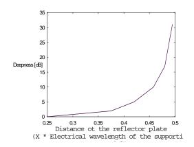
Fig.8 Deepness of the radiation pattern vs. distance of the reflector for omnidirectional antenna with circular polarization
