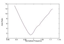
Fig.10b Simulated axial ratio vs. frequency for omnidirectional antenna with circular polarization and conical radiation pattern
