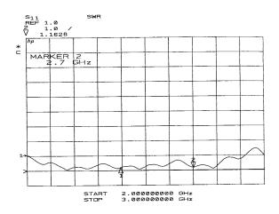
Fig.4c Measured VSWR of antenna with beam width of 180<sup>0</sup> In azimuth plane
