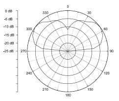
Fig.11a Measured radiation pattern for omnidirectional antenna with circular polarization and conical radiation pattern
