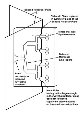
Fig.3 Side outlook of the antenna structure with beam width of 180<sup>0</sup> in azimuth plane
