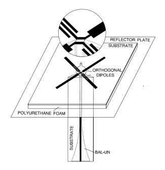
Fig.7 Two orthogonal dipoles fed by balanced (symmetrical) microstrip which form antenna for circular polarization
