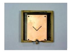
Fig.12b V-slot antenna prototype for circular polarization
