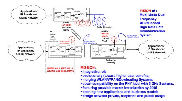
Fig.1d Vision of 60 GHz communication system as evolution of current WLAN and WPANs in 5 GHz range, allowing their next generation. The system is able to operate in both RF and IF range according to preferences
