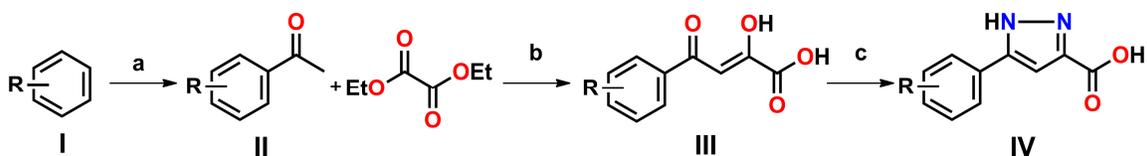
**Scheme 1.** Synthesis of 5-aryl-1*H*-pyrazole-3-carboxylic acids. (a)  $\text{CH}_3\text{COCl}$ ,  $\text{AlCl}_3/\text{CH}_2\text{Cl}_2$ , 6h,  $0^\circ\text{C}$  to rt; (b) 2 eq.  $\text{Na}/\text{CH}_3\text{OH}$ ,  $15^{\text{h}}$ , rt, then conc.  $\text{HCl}$ , (c)  $\text{N}_2\text{H}_4 \cdot \text{H}_2\text{O}/\text{CH}_3\text{COOH}$ ,  $8^{\text{h}}$ , rt.
