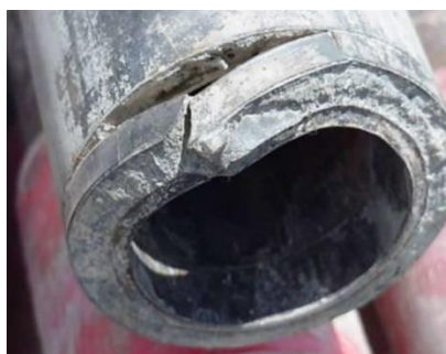
Figure 4. Degradation of oil and gas pipelines under acid corrosion
