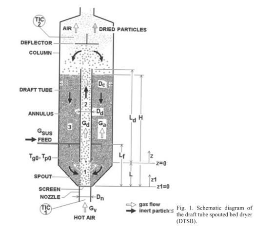
high moisture content (suspensions, sludges, *etc.*) can be dried in a single step, with the process working continuously.
