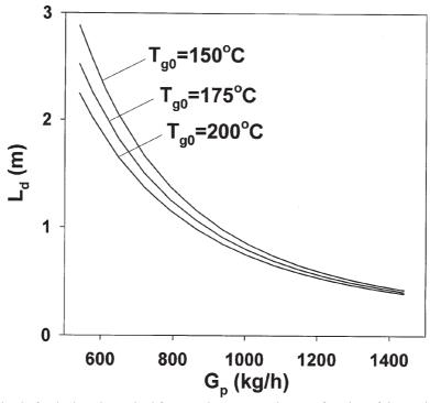
Fig. 2. The draft tube length required for complete evaporation as a function of the particle circulation rate and the inlet air temperature ( $G_v = 306 \text{ kg/h}$ ;  $G_d = 265 \text{ kg/h}$ ;  $G_a = 41 \text{ kg/h}$ ;  $T_{p0} = 73 \text{ °C}$ ; feed-water,  $G_{SUS} = 12 \text{ kg/h}$ ).
