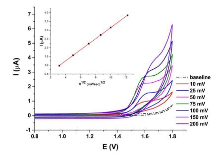
**Figure 3.** Cyclic voltammograms of 0.1 mM of clomazone at BDD electrode (working electrode) and Ag/AgCl electrode (reference electrode) in BRBS at pH 2 at various scan rates from 10 to 200 mV/s. Inset figure present dependence of the peak current from the square root of the scan rate.
