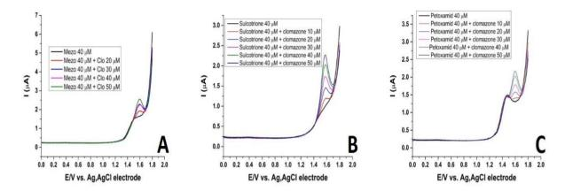
**Figure 6.** Electrochemical response of clomazone in the presence of some tested interferences by SWV method: A) mezotrione; B) sulcotrione; C) pethoxamid. BDD as working electrode, Ag/AgCl electrode as reference electrode, supporting electrolyte BRBS at pH 2. Pulse amplitude 40 mV, frequency 20 Hz.
