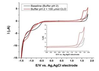
**Figure 1.** Cyclic voltammogram of 0.1 mM of clomazone in BRBS at pH 2 with BDD as working electrode and Ag/AgCl electrode as reference electrode. Scan rate 100 mV/s. Insert figure shown electrochemical response of 0.1 mM clomazone in anodic range potential.
