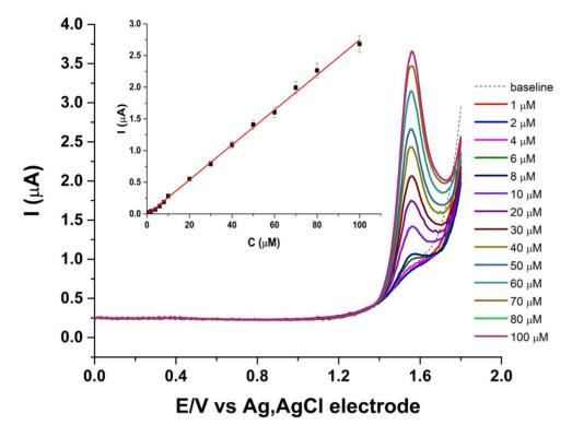
**Figure 5.** Voltammograms obtained for different concentrations of clomazone in positive potential range. SWV technique, working electrode BDD, reference electrode Ag/AgCl electrode, supporting electrolyte BRBS (pH 2). Pulse amplitude 40 mV, frequency 20 Hz. Insert figure shown corresponding calibration curve.
