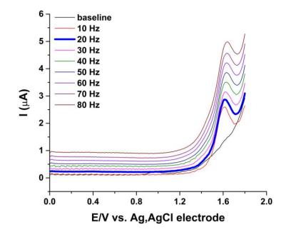
**Figure 4.** Optimization of the SWV frequency in the range from 10 to 80 Hz of 0.1 mM of clomazone at BDD electrode as working electrode and Ag/AgCl electrode as reference electrode in BRBS at pH 2. Pulse amplitude 40 mV.
