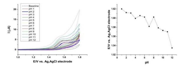
**Figure 2.** Cyclic voltammograms of 0.1 mM of clomazone at BDD (working) electrode and Ag/AgCl (reference) electrode in various pHs of supporting electrolytes. Scan rate 100 mV/s. Dependence of the peak potential against pH values.
