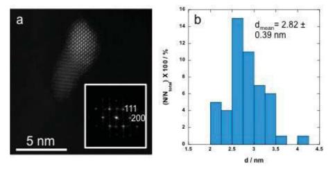
Figure 3. a) High resolution transmission electron micrograph (HRTEM) along with FFT (in inset) with noted 111 and 200 reflections and b) particle size distribution of PtAu/C catalyst with the calculated mean particle size of 2.82±0.39 nm
