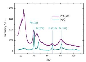
Figure 1. XRD patterns of PtAu/C and Pt/C catalysts Slika 1. XRD dijagrami za PtAu/C i Pt/C katalizatore
