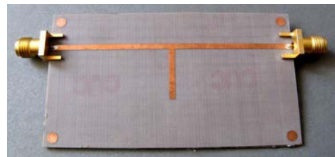
Fig. 8. Photo of the upper side of the fabricated microstrip sensor
