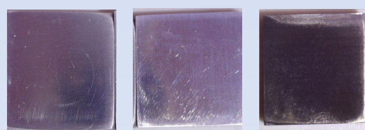
Figure 4. Optical Microscope picture of metal specimen in a) 0.1M NaCl + 3mM cysteine, b) 0.1M NaCl + 3mM complex, c) 0.1M NaCl.
