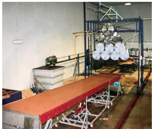
View of the nozzle spray rainfall simulator and soil flume. The installation includes attributes to simulate wind-driven rain.
