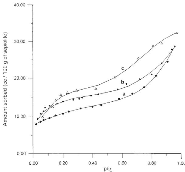
Fig. 7. Adsorption isotherms of: a) methanol, b) ethanol, and c) *n*-butanol on the Goleš sepiolite.
