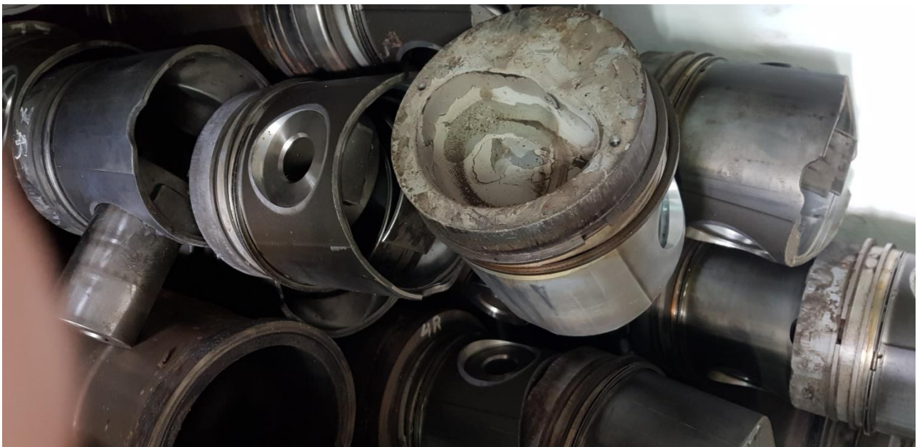
Figure 3: Example of damaged and replaced pistons due to impurities in LFG and silica deposits
