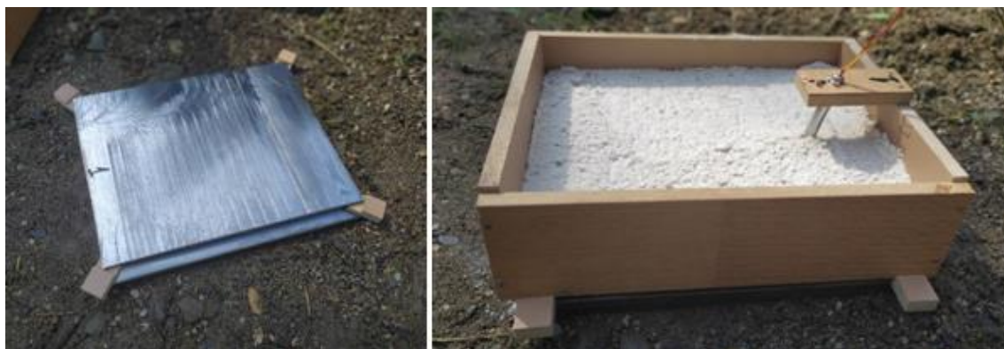
Figure 3. Experimental set-up for explosion welding, left: steel plates in parallel configuration with wooden spacers; right: wooden frame placed over the plates with DEMEX explosive and blasting cap placed in a holder
