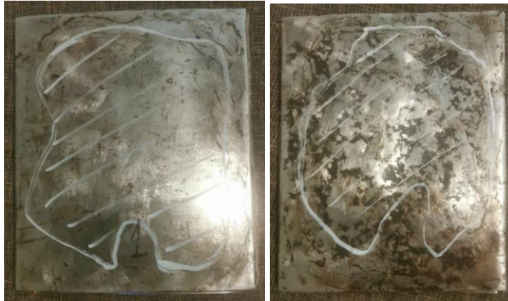
Figure 4. Explosively welded plates 1 and 2: area of weld, registered by ultrasonic method
