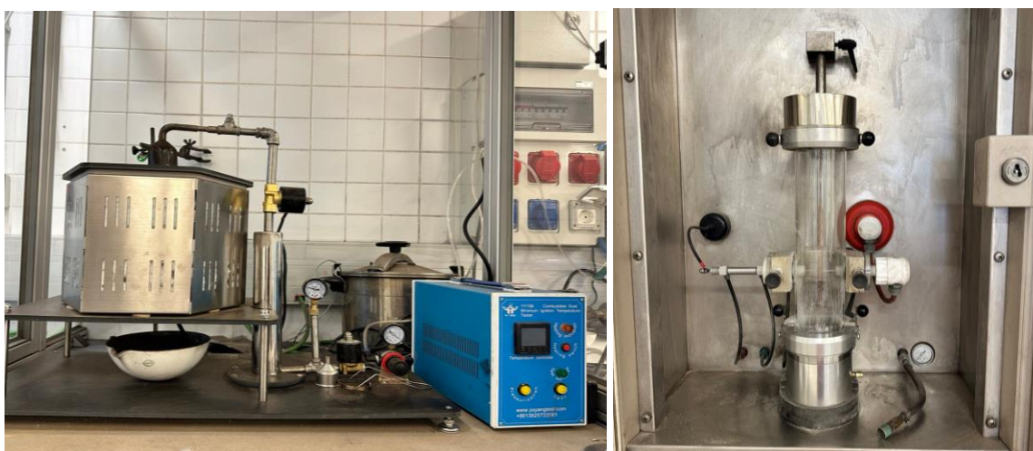
Figure 1: G-G furnace for MITc determination (left) and MIKE 3 apparatus for MIE determination (right)
