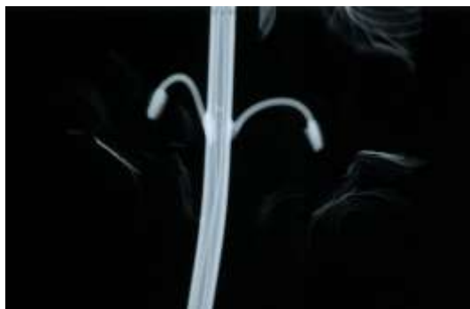
Figure 3. Negative of X-ray film at central part of desk lamp with leaves ( \approx 1\text{mm} in thickness) [9]
