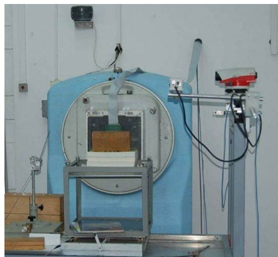
Figure 5. The radiation unit IRPIK-B at the Metrology Dosimetry Laboratory of the Vinča Institute of Nuclear Sciences, used for \gamma -irradiation of the samples
