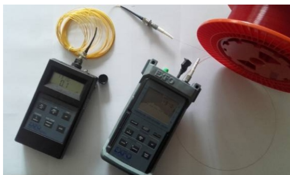
Figure 3. The principle scheme of insertion loss measurements in optical connectors by the EXPO FOT-900 single mode Fibre Optic Test System instrument
