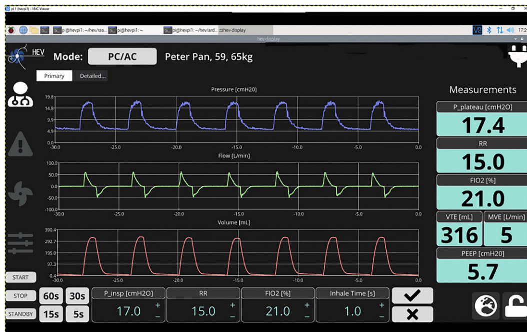
Figure 4. Example home screen display from the native user interface. Numbers and graphs are indicative.
