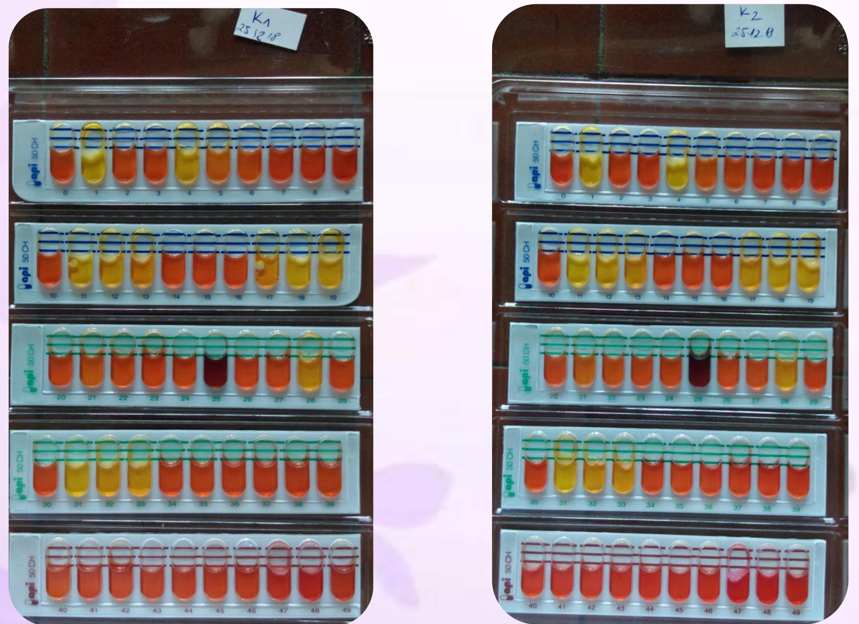
Figure 1. The results of the API 50CHB / E test for two colonies K1 (left) and K2 (right).
