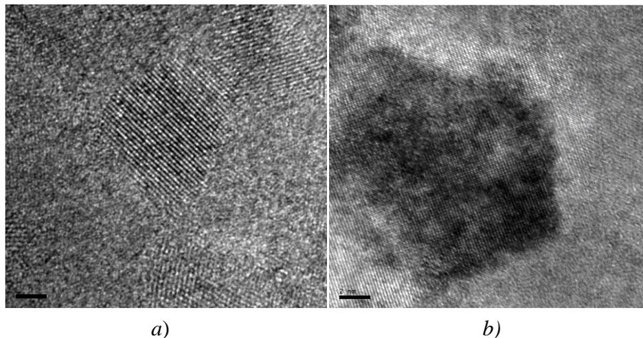
*Fig. 5 – HREM images of a) Nd-low and b) Nd-rich alloy in the optimal magnetic state*
