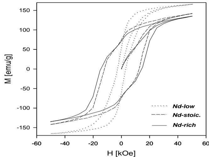
Fig. 6 - Hysteresis loops of investigated Nd-Fe-B alloys in optimized magnetic state
