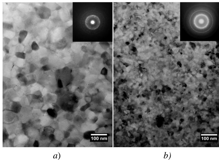
*Fig. 4 – TEM images of a) Nd-low and b) Nd-rich alloy in the optimal magnetic state*
