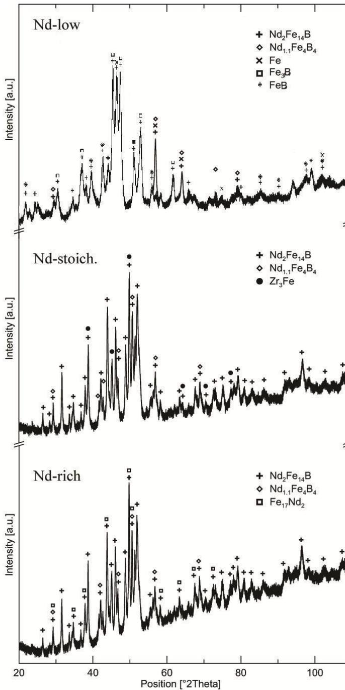
Fig. 2 – X-Ray diffractograms of the investigated alloys
