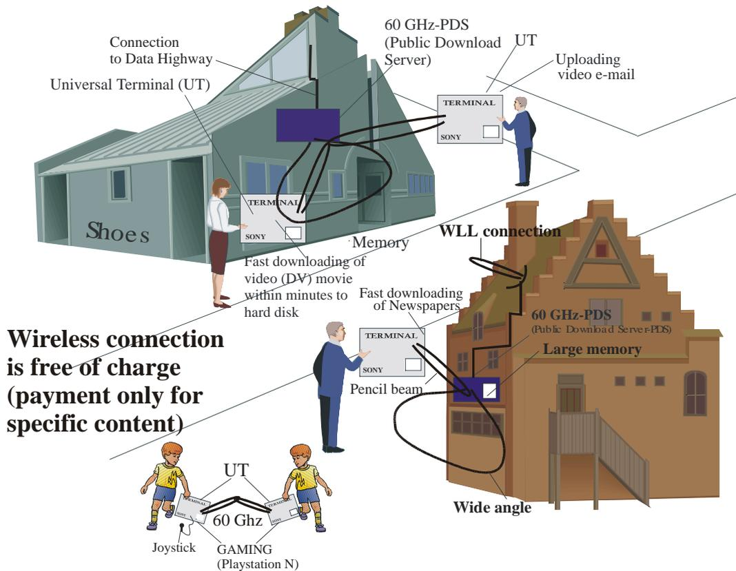
Fig.1b Possible out-door application scenario for fast downloading and uploading and free of charge broadband internet in urban areas
