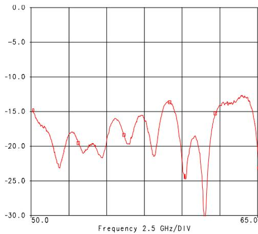
Fig.2b Measured input reflection loss of linear polarized high gain antenna array for 60 GHz range
