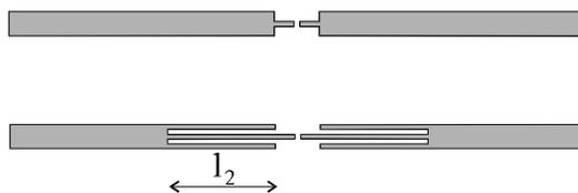
Fig.6 Pair of dipoles with conjugated impedances
