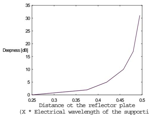
Fig.8 Deepness of the radiation pattern vs. distance of the reflector for omnidirectional antenna with circular polarization
