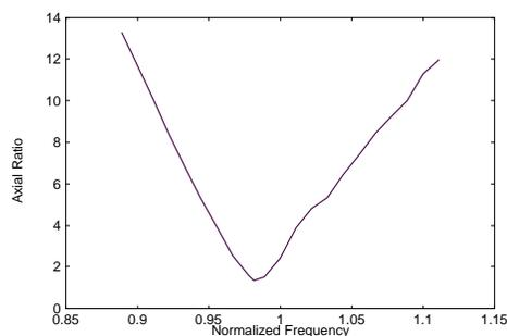
Fig.10b Simulated axial ratio vs. frequency for omnidirectional antenna with circular polarization and conical radiation pattern
