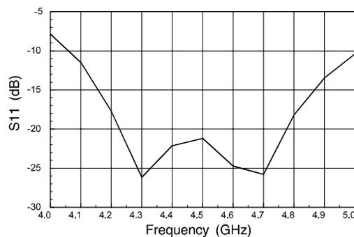
Fig.10a Simulated  $S_{11}$  vs. frequency for omnidirectional antenna with circular polarization and conical radiation pattern
