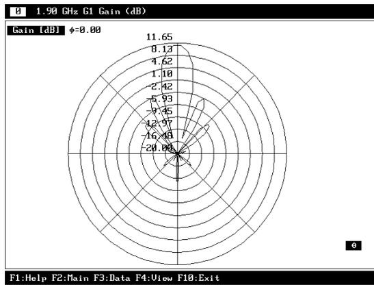
Fig.4b Simulated antenna diagram in elevation plane, dBi (no loss)
