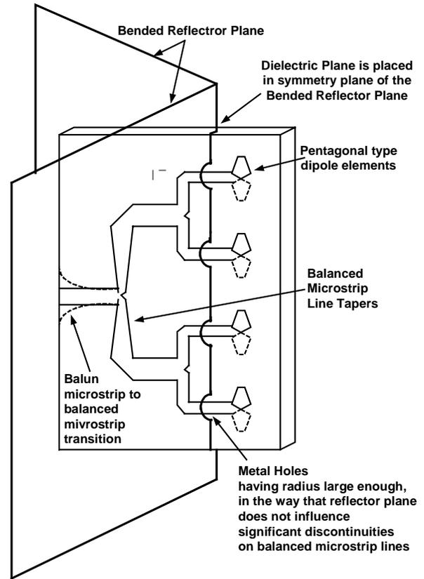
Fig.3 Side outlook of the antenna structure with beam width of  $180^\circ$  in azimuth plane
