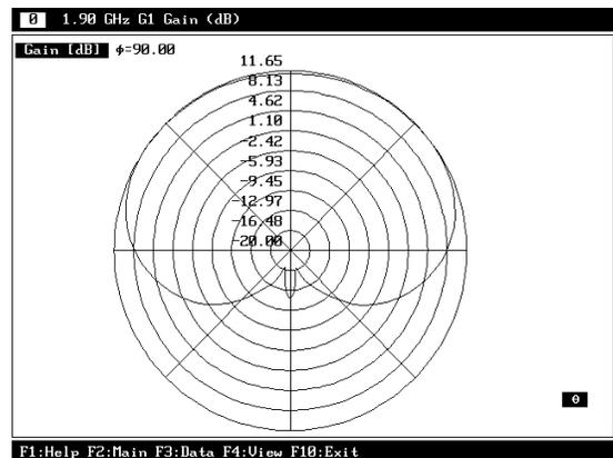
Fig.4a Simulated antenna diagram in azimuth plane, dBi (no loss)
