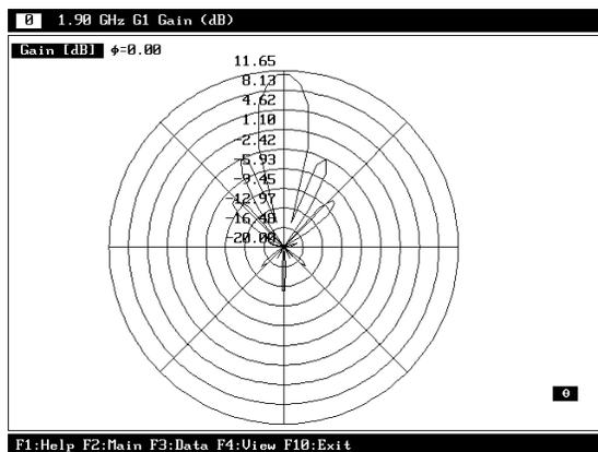
Fig.4b Simulated antenna diagram in elevation plane, dBi (no loss)
