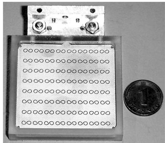
Fig.14 Antenna array with 8x8 slot radiating elements with circular polarization for 60 GHz band
