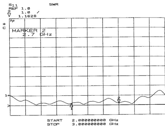
Fig.4c Measured VSWR of antenna with beam width of 180° In azimuth plane
