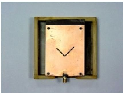
Fig.12b V-slot antenna prototype for circular polarization
