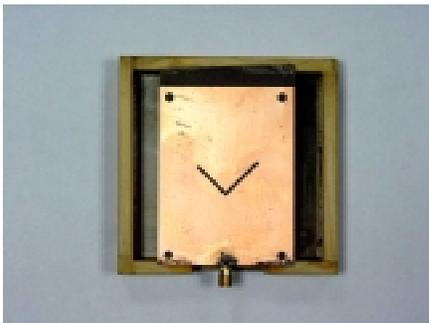
Fig.12b V-slot antenna prototype for circular polarization
