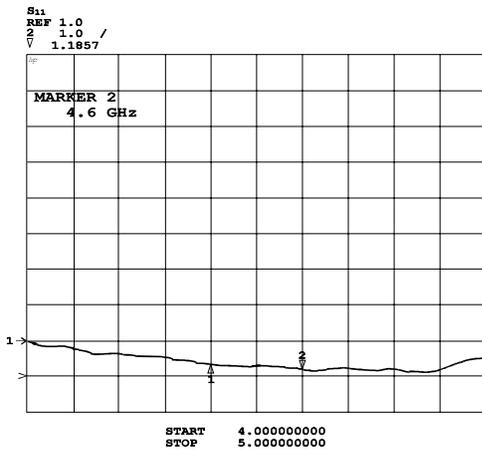
Fig.11b Measured VSWR vs. frequency for omnidirectional antenna with circular polarization and conical radiation pattern
