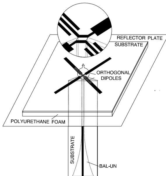
Fig.7 Two orthogonal dipoles fed by balanced (symmetrical) microstrip which form antenna for circular polarization
