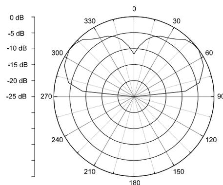
Fig.11a Measured radiation pattern for omnidirectional antenna with circular polarization and conical radiation pattern
