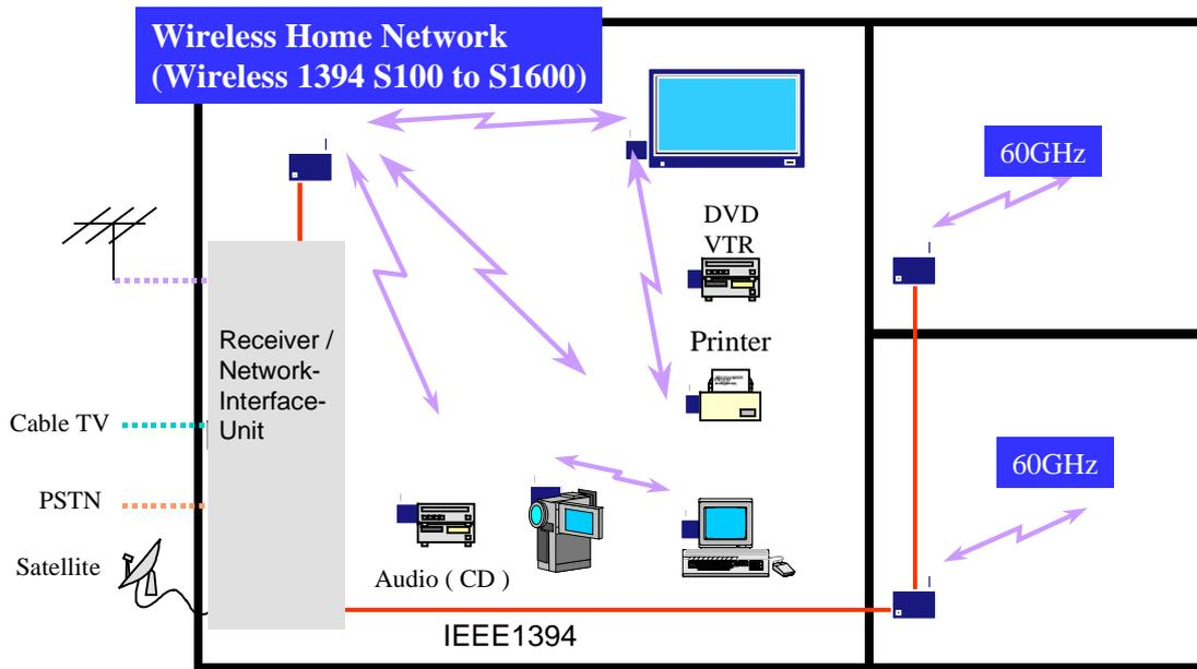
Fig.1a Possible in-door home application scenario for both analog and digital application
