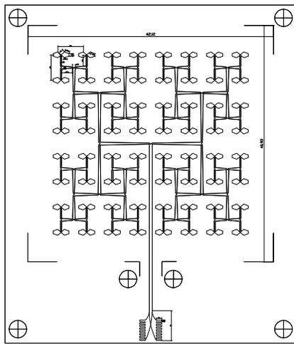
Fig.2a Projection of the linear polarized high gain antenna array prototype prints for 60 GHz range
