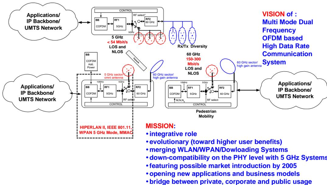
Fig.1d Vision of 60 GHz communication system as evolution of current WLAN and WPANs in 5 GHz range, allowing their next generation. The system is able to operate in both RF and IF range according to preferences
