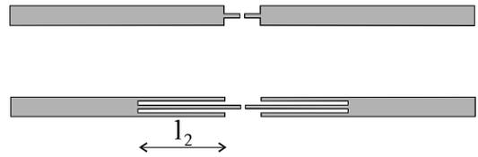
Fig.6 Pair of dipoles with conjugated impedances
