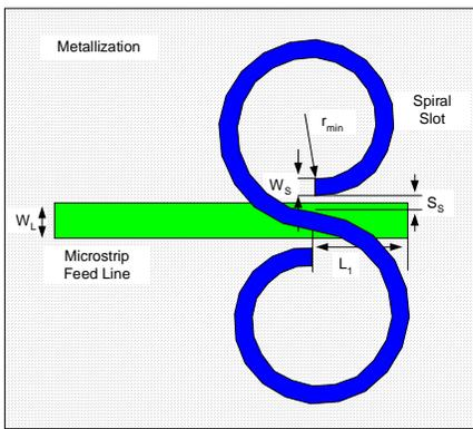
Fig.12a Spiral slot antenna prototype for circular polarization
