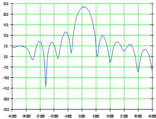
Fig.2c Measured antenna diagram (60 GHz), dBi
