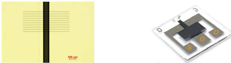
Fig. 2. (a) Optical micrograph the nanochannel array etched in a Pyrex substrate; (b) Photo of an assembled device, chip dimensions 1 x 1 cm. The transistor gate (top) is electrostatically bonded to the Pyrex substrate covering the nanochannels array. Contact pads are denoted by S for the source, G for the gate and D for the drain, respectively.
