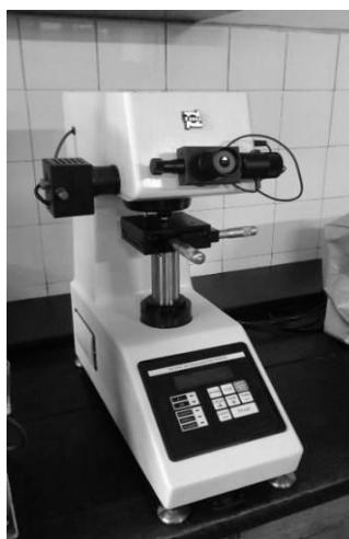
Slika 5.6 Micro Vickers Hardness Tester: TH710 [162]
