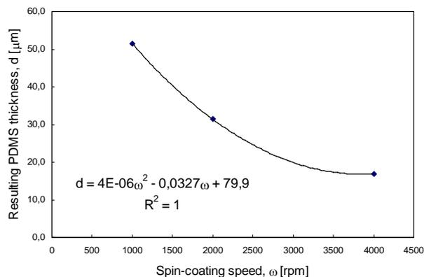
**Picture 2:** Dependence of the PDMS layer thickness as a function of spin speed for a rotation time 60 s (5 s 500 rpm + 55 rpm).
