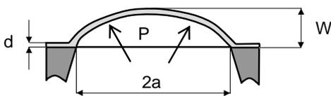
**Picture 6.:** Schematic diagram of the membrane with a uniform pressure applied to one side.
