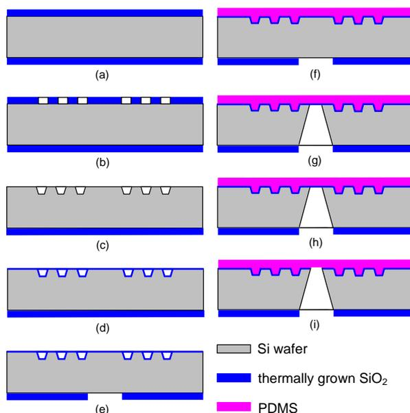
**Picture 1:** Fabrication sequence of cavity coated with PDMS membrane. Structure is fabricated by bulk micromachining on {100} oriented Si wafers with cavity edges oriented in  $\langle 110 \rangle$  direction.
