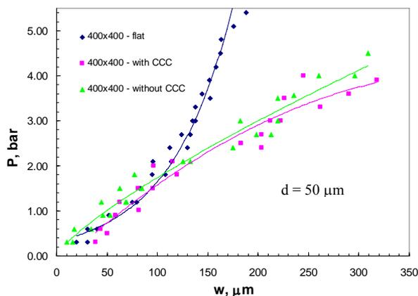
**Picture 10.** Experimental results on the measured maximum deflection ( $w$ ) as a function of applied pressure ( $P$ ) for square membrane with  $400 \times 400 \mu\text{m}^2$  dimensions and  $50 \mu\text{m}$  PDMS thickness for membranes fabricated on flat Si substrate, and Si substrates with purposely made corrugations with or without convex corners compensations
