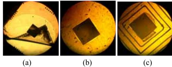
**Picture 8.** Photographs from microscope (first is under two times smaller magnification) of  $400 \times 400 \mu\text{m}^2$  PDMS membranes  $50 \mu\text{m}$  thick, after they lost adhesion with substrate under the applied pressure.
