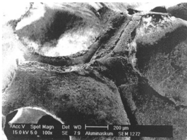
Fig. 6. SEM Micrograph of the porous ceramic obtained by repeated immersion and drying processes.
