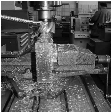
Figure 1 Copper anode mechanical finishing
