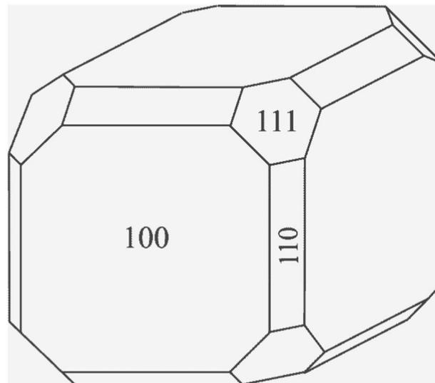
**Fig. 4** A crystal with a simple cubic lattice and (100), (111) and (110) faces. (According to ref. 32).
