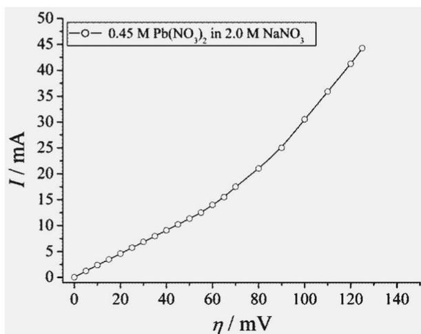
Fig. 1 The polarization curve for lead electrodeposition from 0.45 M Pb(NO<sub>3</sub>)<sub>2</sub> in 2.0 M NaNO<sub>3</sub>. The surface area of the copper working electrode = 0.25 cm<sup>2</sup>.
