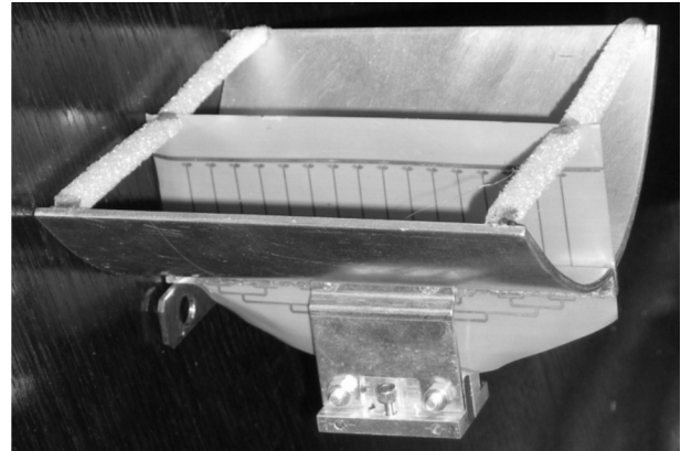
Figure 9: Photograph of the realized 60 GHz antenna array (D) in the cylindrical-parabolic reflector with uniform feed distribution.
