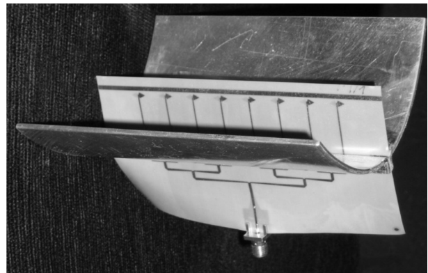
Figure 6: Photograph of the realized 26 GHz antenna array (A) in the cylindrical-parabolic reflector with uniform feed distribution.
