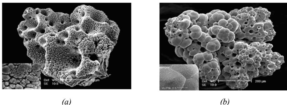
Fig. 4. SEM microphotographs of cobalt powder particles deposited at  $j_{L(Co)} = 770 \text{ mA cm}^{-2}$  onto cobalt electrode; (a) agglomerate, (b) spongy-like particle, with details of their surface.
