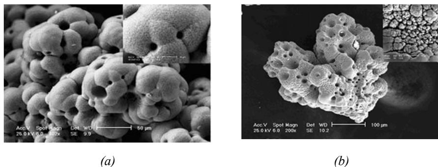
Fig. 3 SEM microphotographs of cobalt powder particles deposited at  $j_{L(\text{Co})} = 770 \text{ mA cm}^{-2}$  onto glassy carbon electrode; (a) the agglomerate and detail of surface, (b) spongy-like particle with detail of surface.
