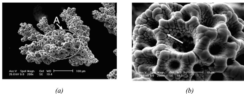
Fig. 5. SEM microphotographs of cobalt powder particles deposited at  $j_{L(Co)} = 770 \text{ mA cm}^{-2}$  onto nickel electrode; (a) spongy-like cobalt powder particles, (b) details of (A) spongy-like particle.
