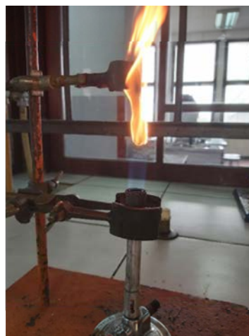
Figure 7. Standard and laboratory setup of apparatus (right) for vertical testing of thermal stability of samples [10]
