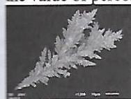
Figure Left: Galvanostatically electrodeposited copper powder Figure Right: Electrical conductivity of composites
