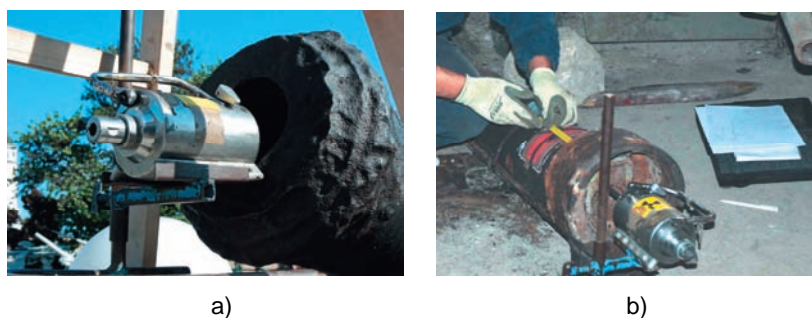
Figure 3. Radiographic recording a) barrel of the French ship cannon, AN 1808 RUELLE, b) barrel of the French cannon 75/27 model 1911 Deport (Military Museum in Kalemegdan in Belgrade)
