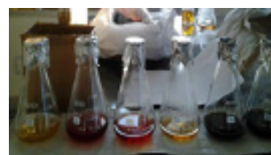
Fig. 1: Color change of biomass samples treated at different temperature: 200°C (left) and 300°C (right) (Song and Kim, 2013)
