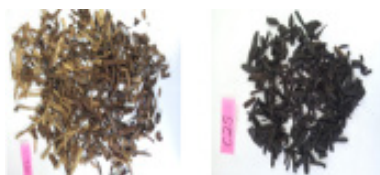
Fig. 1: Color change of biomass samples treated at different temperature: 200°C (left) and 300°C (right) (Song and Kim, 2013)
