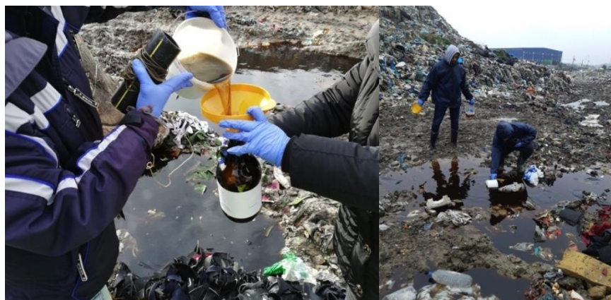
Figure 1. Collecting of leachate at a non-sanitary municipal solid waste landfill in Novi Sad in winter (left) and spring (right) 2019
