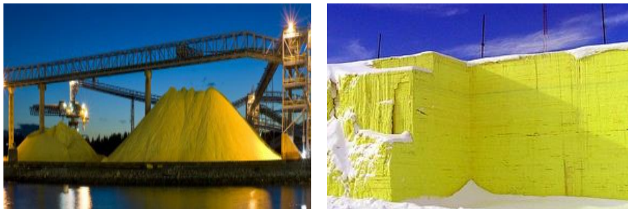
Figure 2. Piles [3] and blocks [4] of sulfur produced by Claus process
