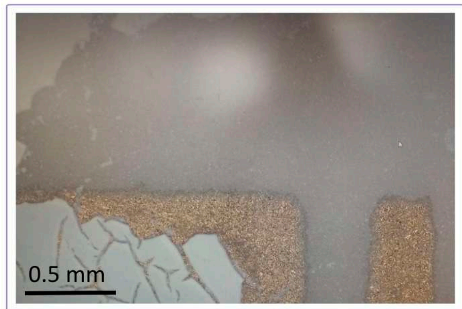
Figure 6. Peeling off of the TiO 2 layer from the substrate edges.
