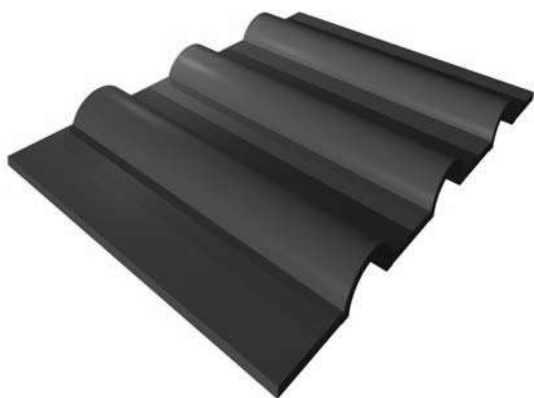
Fig. 1. General presentation of a sculpted nanomembrane with a diffractive grating formed by an array of reversed troughs with ellipsoidal profiles.
