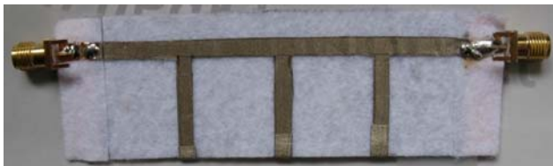
Figure 5: Structure with conductive textiles from above.
