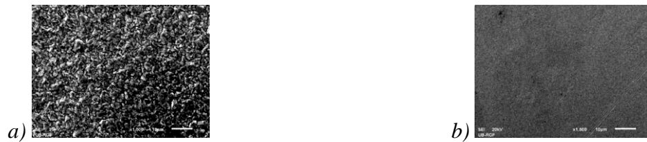
Figure 5. The morphology of 20 \mu\text{m} thick Cu coatings on brass substrate obtained by electrodeposition (DC/MS regime) at a current density of 50 \text{ mA cm}^{-2} on the brass from: (a) electrolyte I, and (b) electrolyte II. Magnification: \times 1500 [3].
