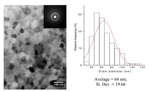
Fig. 3 Bright field TEM micrograph of Nd<sub>14</sub>Fe<sub>79</sub>B<sub>7</sub> alloy in optimal magnetic state with grain size distribution
