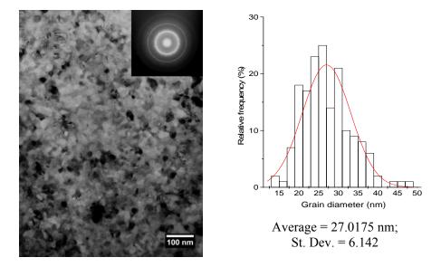
Fig. 2 Bright field TEM micrograph of Nd<sub>4.5</sub>Fe<sub>77</sub>B<sub>18.5</sub> alloy in optimal magnetic state with grain size distribution
