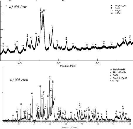
**Fig. 1** X-ray diffraction patterns of the investigated Nd<sub>4.5</sub>Fe<sub>77</sub>B<sub>18.5</sub> and Nd<sub>14</sub>Fe<sub>79</sub>B<sub>7</sub> alloys in optimized magnetic state: a) Nd-low alloy; b) Nd-rich alloy
