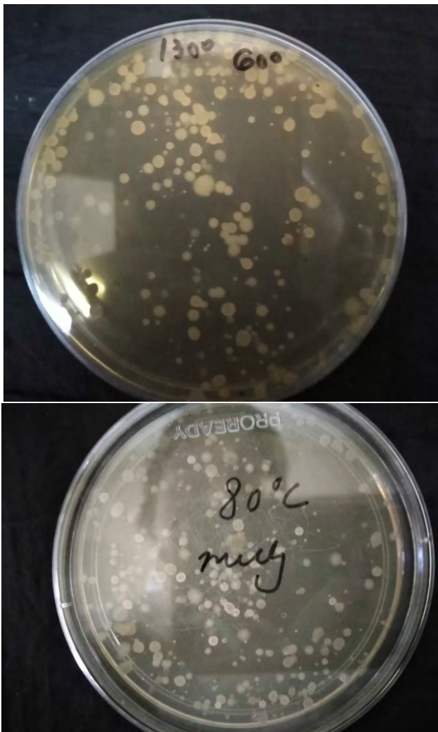
Figure 7: Microorganisms viability after fluidized bed drying at 60 and 80 °C
