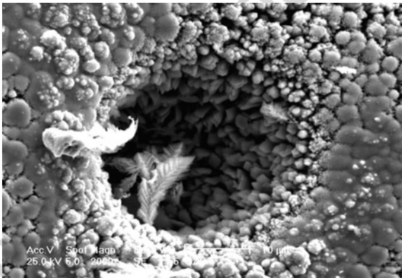
Fig. 2.31 SEM micrograph of the cavity detected on the ball-like agglomerate (Reprinted from [99] with the permission of Springer-Verlag.)
