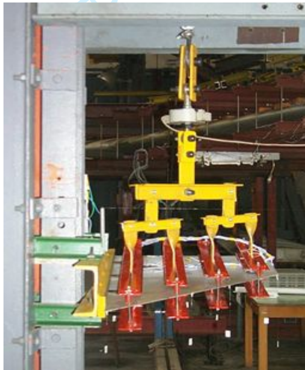
Fig. 3 The experimental installation for static test of the real-sized fin model
