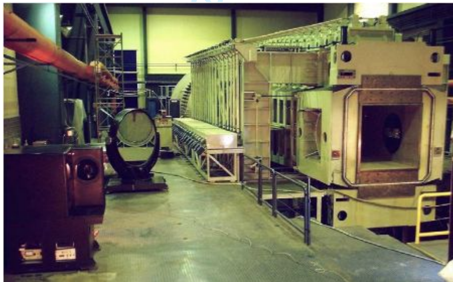
Fig. 2 a) The T-38 tri-sonic blow-down pressurized test facility with test section
