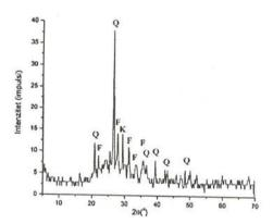
Figure 1. XRD diffractogram of ash dump (Q-quartz, F-feldspar, C-calcite)
